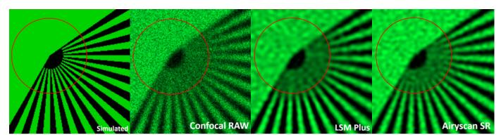
*Figure 11* Resolution limits of Confocal, LSM Plus (Confocal Wiener DCV), and Airyscan SR detection. In addition to the resolution gain, both Airyscan and LSM Plus reduce noise and improve visibility.
