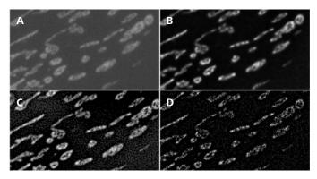
**Figure 17** Example of deconvolution artifacts. A) raw data of mitochondria structures acquired using a widefield fluorescent microscope. B) a good deconvolution example using the constrained iterative method. C) a poor deconvolution example showing invention of structures in the background. D) a poor deconvolution example showing enhanced salt-and-pepper noise and disappearance of structures.
