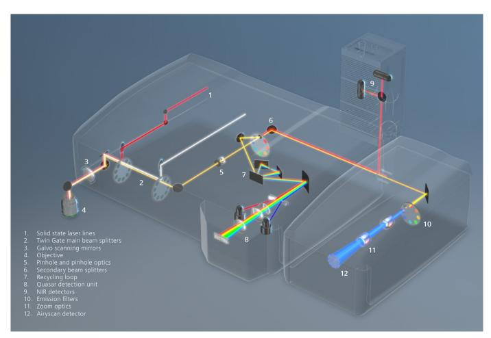
Figure 8 Beam path of LSM 980 with Airyscan 2 and NIR detection
