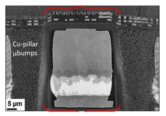
Figure 2c: Backscattered electron SEM image of Cu-pillar microbump (outlined in Fig. 2b) after Ga-FIB polish. Scale bar:  $5 \mu m$ .
