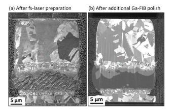
Figure 3: FIB secondary electron image series comparing the cross-section quality directly after fs- laser processing (a) and after an additional Ga-FIB polish step (b). Scale bars:  $5 \mu m$ .
