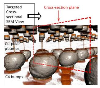
Figure 2a: 3D XRM image of package interconnect consisting of Cu-pillar microbumps and C4 bumps.
