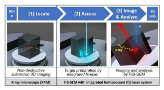
Figure 1: Schematics of the correlative workflow combining 3D XRM (step1), femtosecond laser preparation (step 2), FIB polishing and SEM imaging and analysis (step 3).
