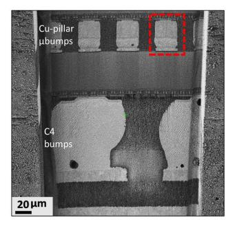
Figure 2b: Backscattered electron SEM image of package interconnect consisting of Cu-pillar microbumps and C4 bumps, immediately after laser processing and correlating to the area defined in Fig. 2a. Scale bar: 20 µm.
